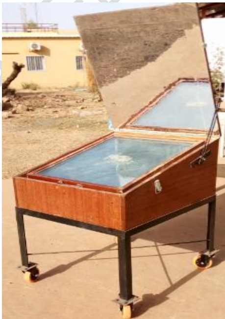
Fig. 1. Picture of the fabricated solar box cooker
