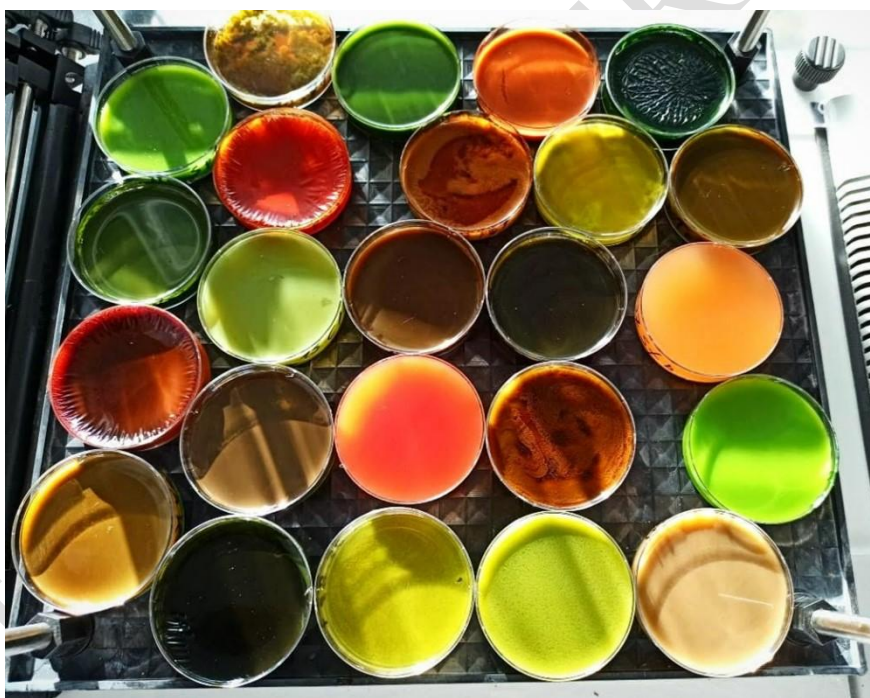
Figure 1. Drying process of aqueous plant extracts using open petri dishes in an incubator shaker at 40°C.
