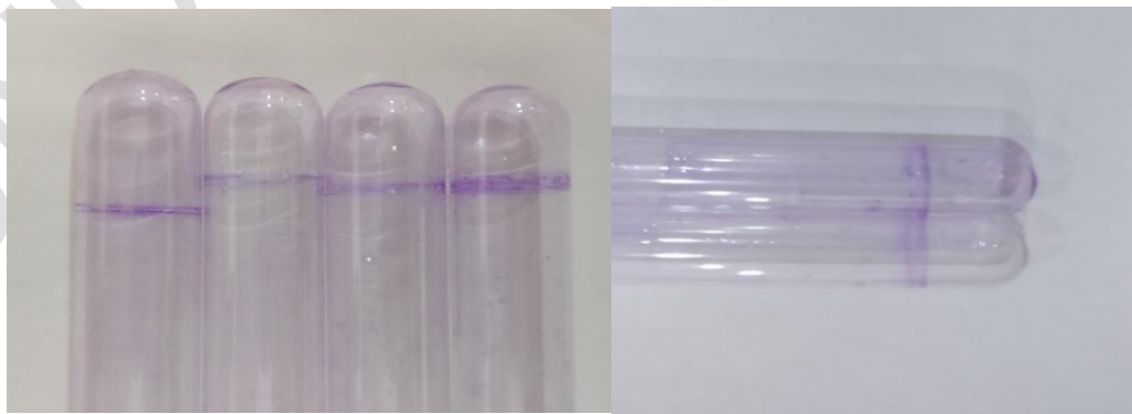
Figure6. Visible film lining the wall and bottom of the tube is indicative of biofilm formation
