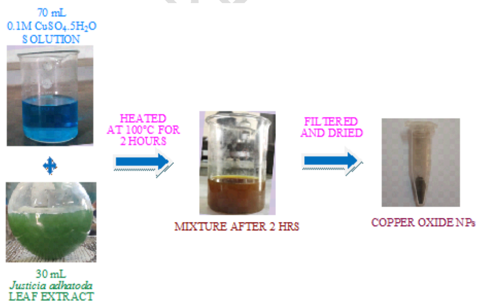
Fig. 3. Biosynthesis of CuO NPs
