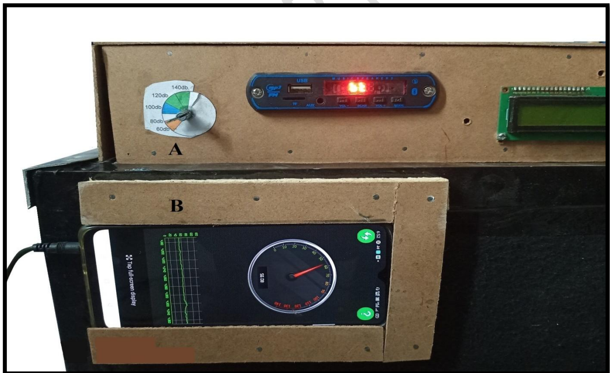
Image 3 showing noise controlling knob with marking (A) and mobile based noise level meter (B)
