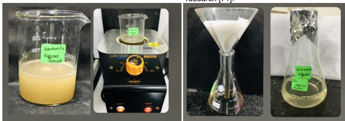
Fig. 1. Preparation of zinc oxide nanoparticle using boerhavia diffusa extract
