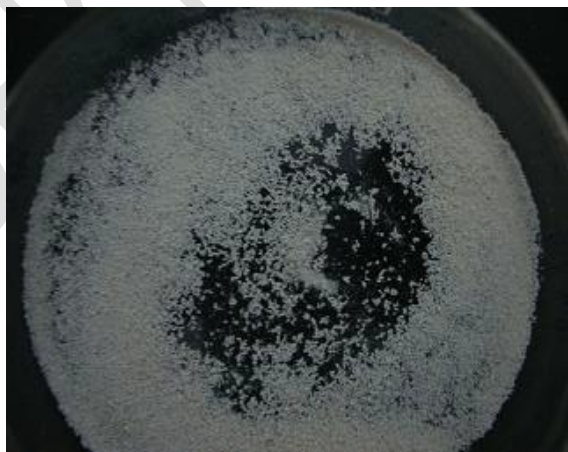
Figure 1: Prepared Rosiglitazone maleate hollow microspheres
