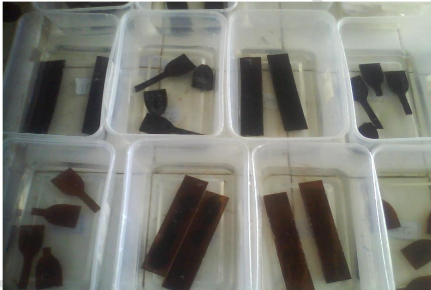
Figure3. Water absorption test
