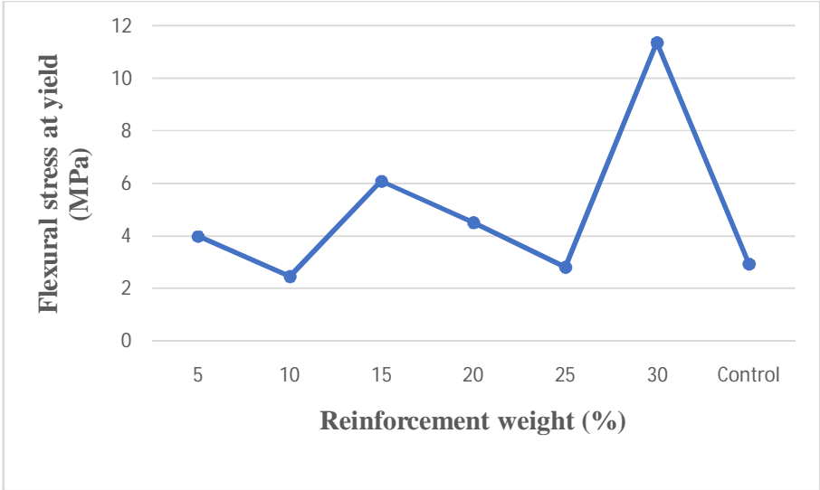
Figure 10. Variation of flexural strength at yield (MPa) with the composite and control
