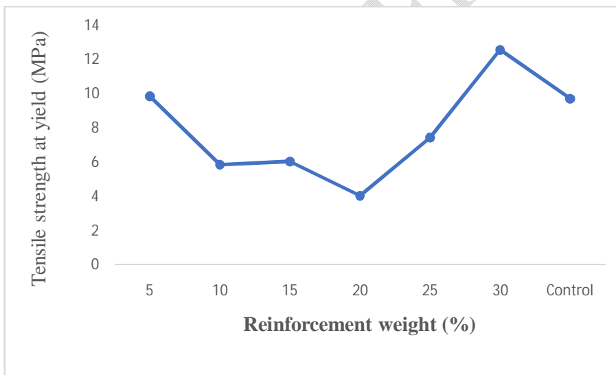
Figure 7. Variation of Tensile strength at yield (MPa) with the composite and control
