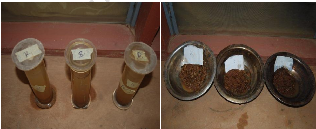
Fig. 12: Specific gravity and Atterberg limit test in progress.
