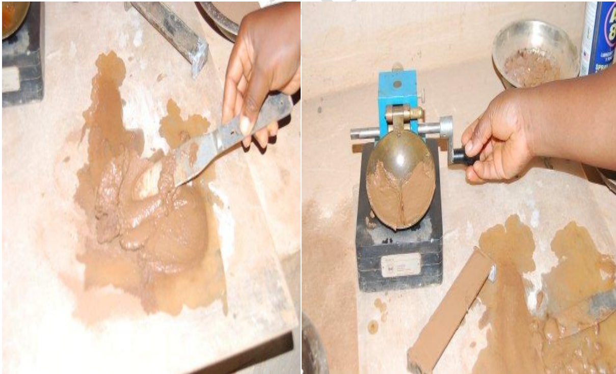
Fig. 13: Atterberg limit test in progress.
