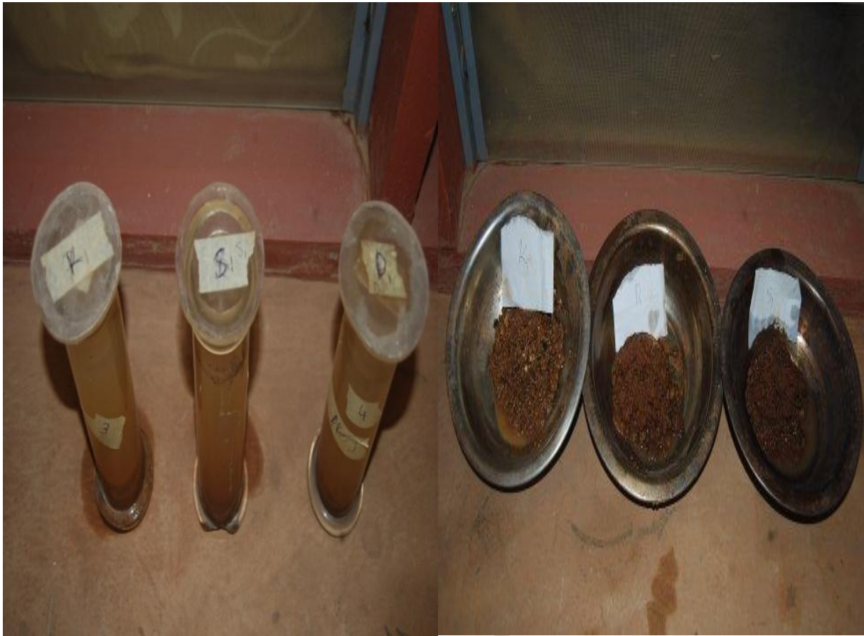
Fig. 12: Specific gravity and Atterberg limit test in progress.
