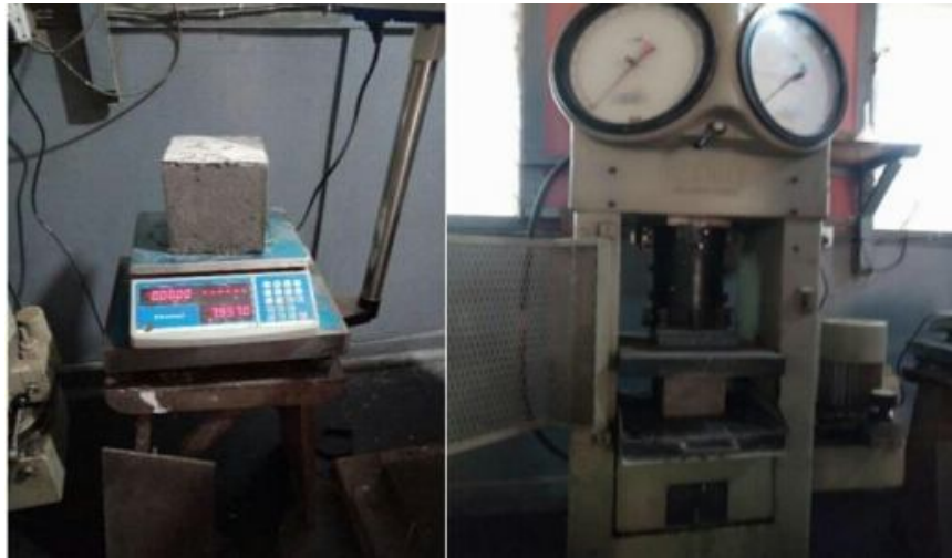
(a) Concrete cube under test
