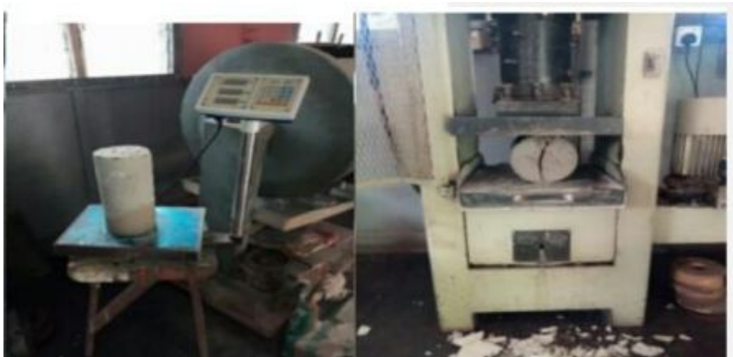
(b) Split concrete cylinder under test
