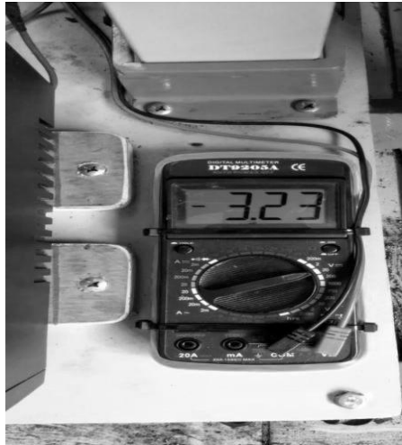
Figure .15 Multimeter voltage output with load (battery)
