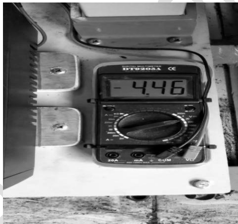
Figure. 16 Multimeter voltage output without Load (Battery)
