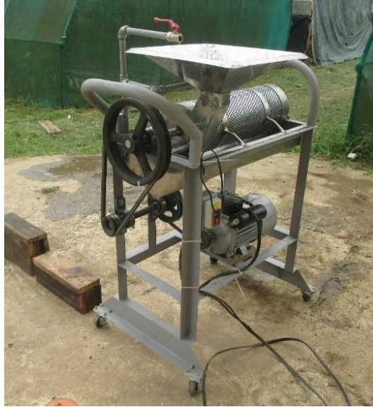
Figure 3. Fabricated demucilaging machine
