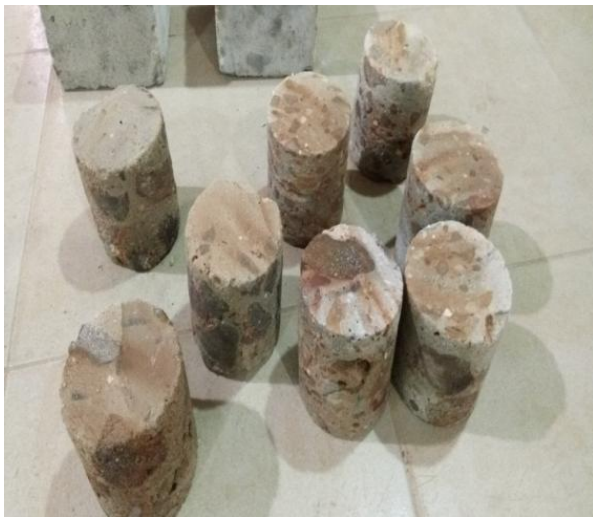
Plate 4: Cored Concrete mass samples.
