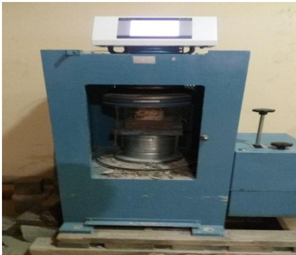
Plate 6: Subjected crushed concrete sample.
