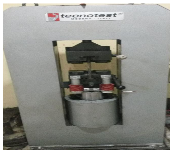
Plate 7: Tensile strength test of reinforcement steel sample.
