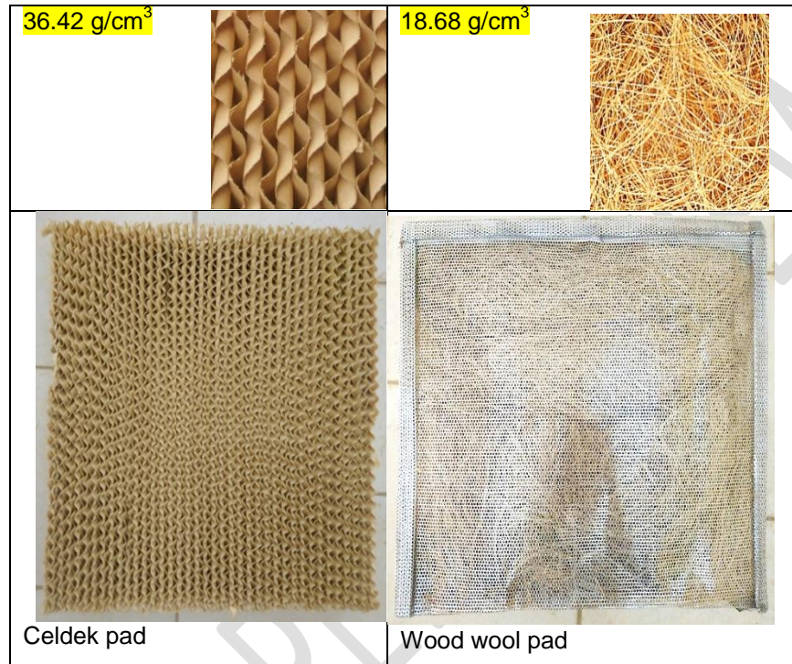
Figure 1 Commercial Celdek pad (left) against locally made wood wool pad (right)
