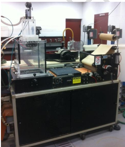
Fig. 3. MK Systems Inc. dynamic sheet former [29]
