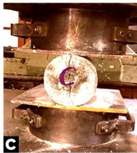
Figure-4 (a,b,c) Test procedure for compressive strength measurement of concrete cylinders
