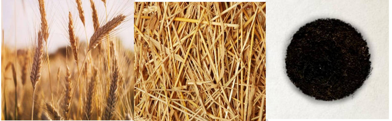
Figure-2 a) Wheat crop b) Wheat Straw separation c) Wheat straw ash burning at 800°C for 30min
