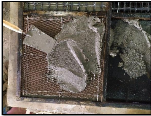
a. shows casting of the bottom skin ferrocement layer
