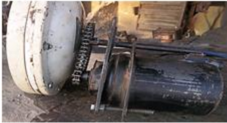
Fig. 4. Wind Turbine Hub and Generator assembly
