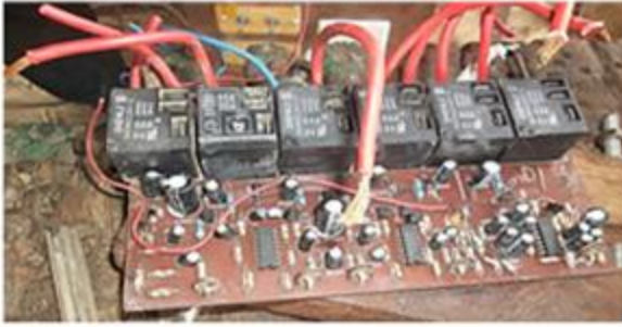
Fig. 2. The Charge Controller
