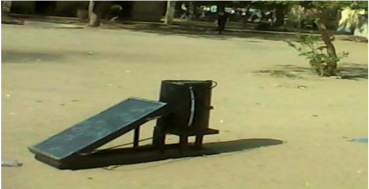
Figure 2: The Constructed Solar Water Heater
