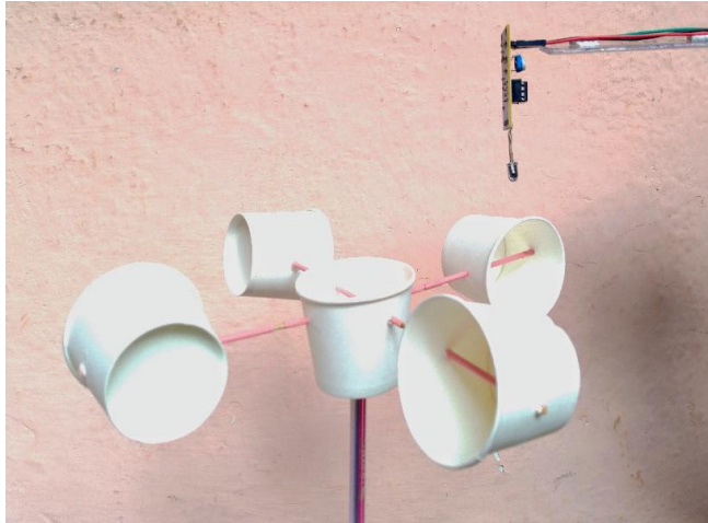
Fig. 15 IR sensor positioned with anemometer
