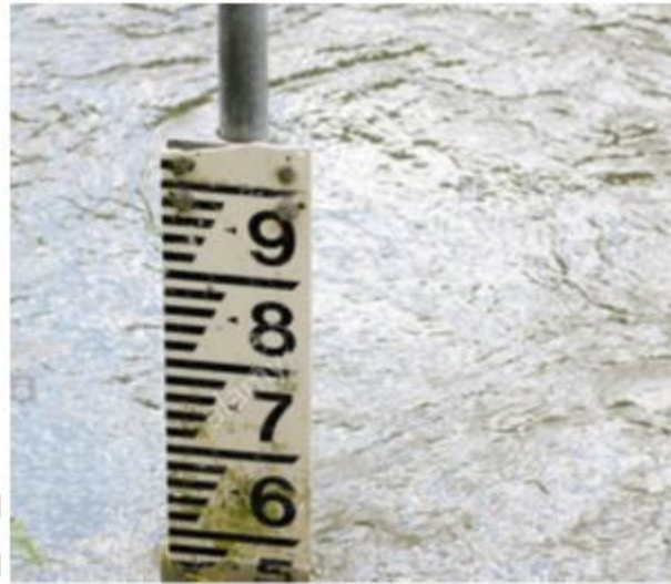
Fig. 9. Measuring canal depth with staff gauge
