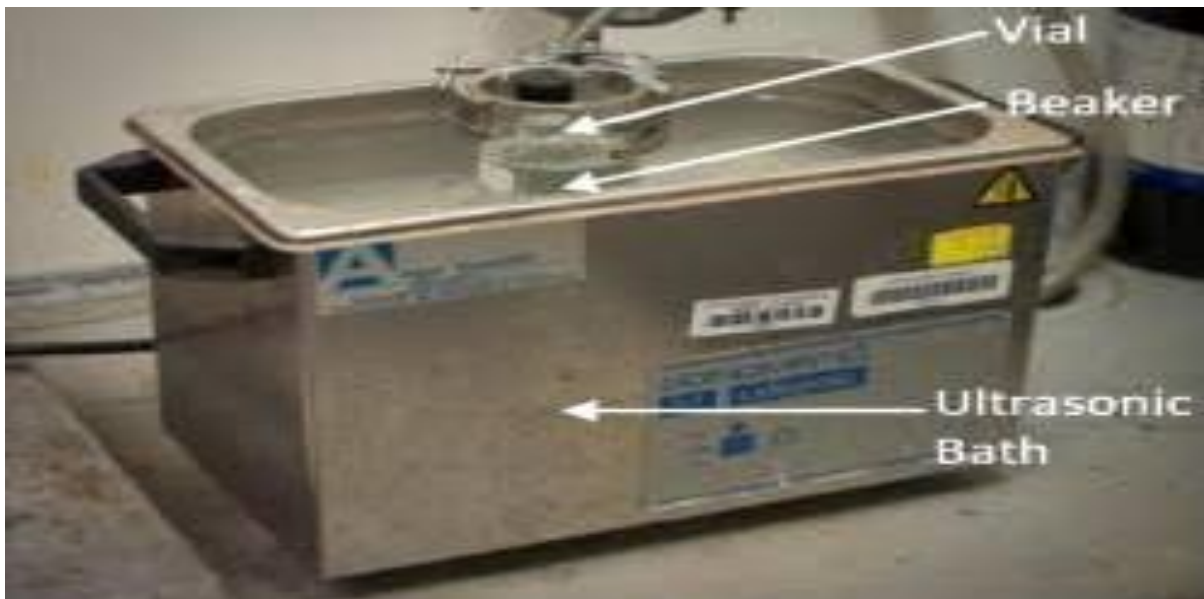
Figure 6: Showing diagrammatical instrumentation of the Sonication bath ( https://www.sciencedirect.com/topic/chemistry/sonication ).
