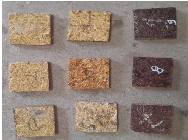
Figure1. Water absorption test specimens
