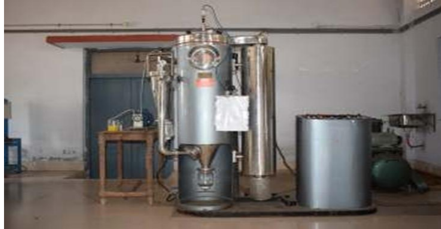
Plate 1. Laboratory model pilot scale spray dryer
