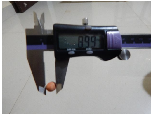
Fig. 1 Measurement of axial dimensions of the groundnut seed
