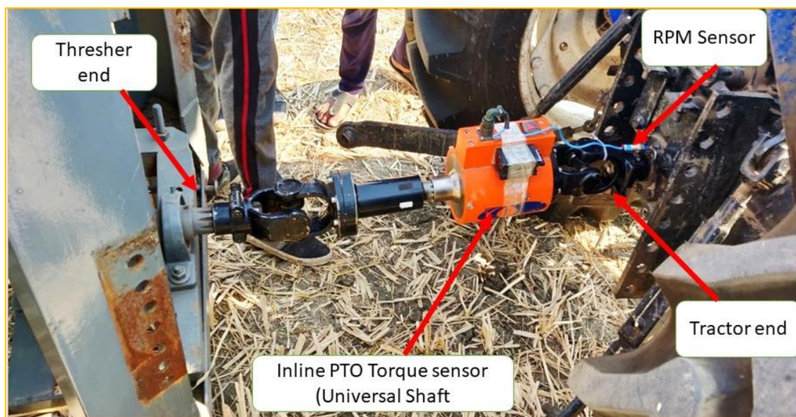
Figure 2 A view of in-line torque sensor
