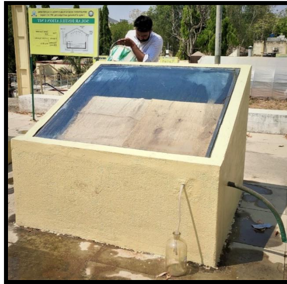
Fig.1. Developed Passive solar distillation unit
