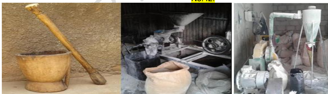
Figure 2: Grinding methods: (A) mortar and pestle; (B) Hammer mill and (C) Disc Mill.
