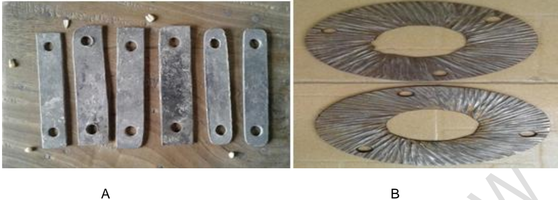
Figure 3: Grinding Machine Discs: (A) Hammer plates; (B) Disc plates
