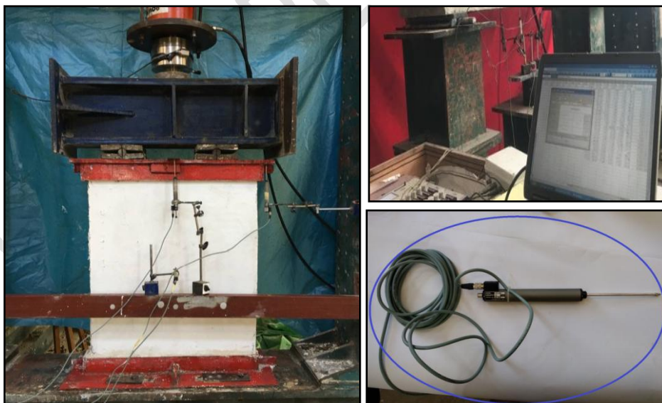
Fig.(15): LVDT sensors, data logger unit and test set up for specimen.
