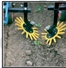
Fig 2: Figure weeder uses rubber spikes that are pointed at an angle towards the crop (Weide et al. 2008)
