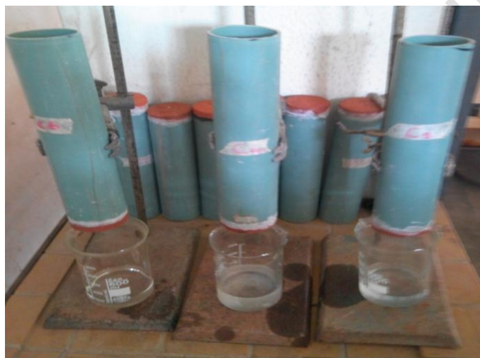
Figure 3: Experimental set up for filtration rate test
