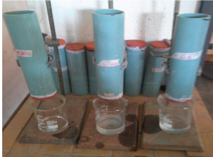
Figure 3: Experimental set up for filtration rate test
