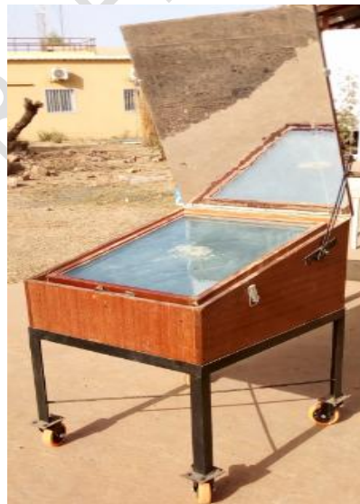
Fig. 1. Picture of the fabricated solar box cooker
