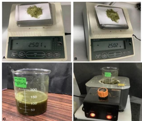
Figure 1: Image A representing 2.5gm of Stevia was measured under the weighing machine. Image B representing 2.5gm of Neem was measured under the weighing machine. Image C representing the Neem and Stevia aqueous formulation and Image D representing aqueous extract of Neem and Stevia boiled for 10-20 minutes at 60 degree Celsius.
