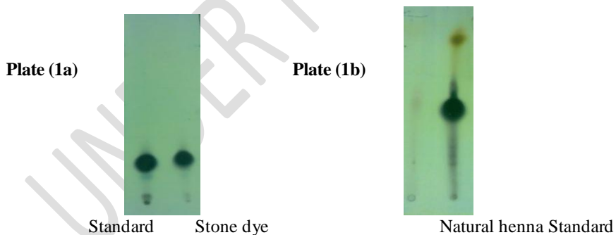
Figure 1: TLC plates (1a, 1b) showed two different solvent systems (Butanol: acetic acid: water & Hexane: Acetone)
