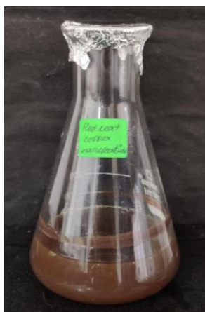
Figure 4: The final reaction solution with red tea mediated copper nanoparticles.
