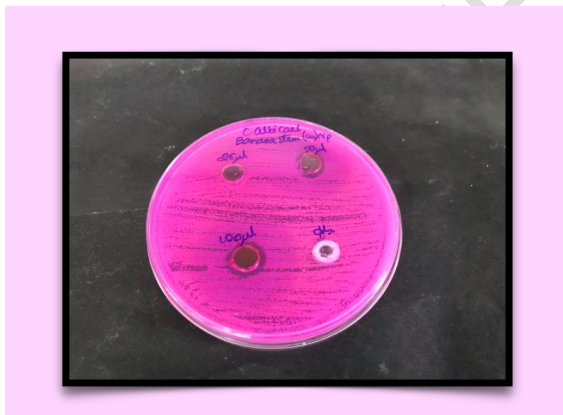
Figure 2 - It shows the zone of inhibition of Candida Albicans which was loaded with different concentrations of musa sapientum mediated copper nanoparticles to check the antimicrobial activity.
