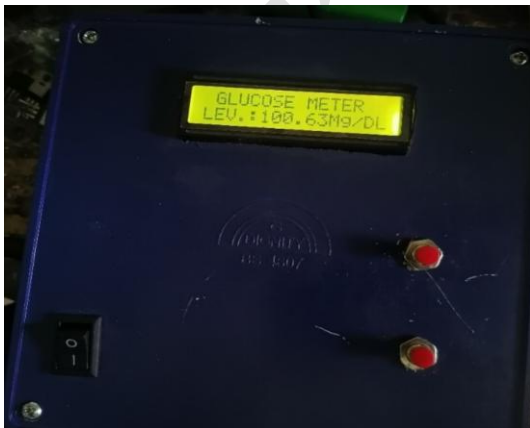
Plate 2: Fabricated Glucometer displaying blood sugar result
