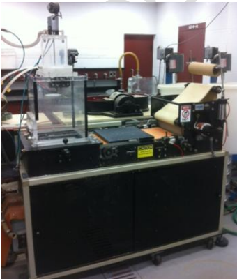
Fig. 3. MK Systems Inc. dynamic sheet former [29]
