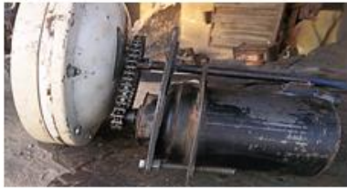
Fig. 4. Wind Turbine Hub and Generator assembly
