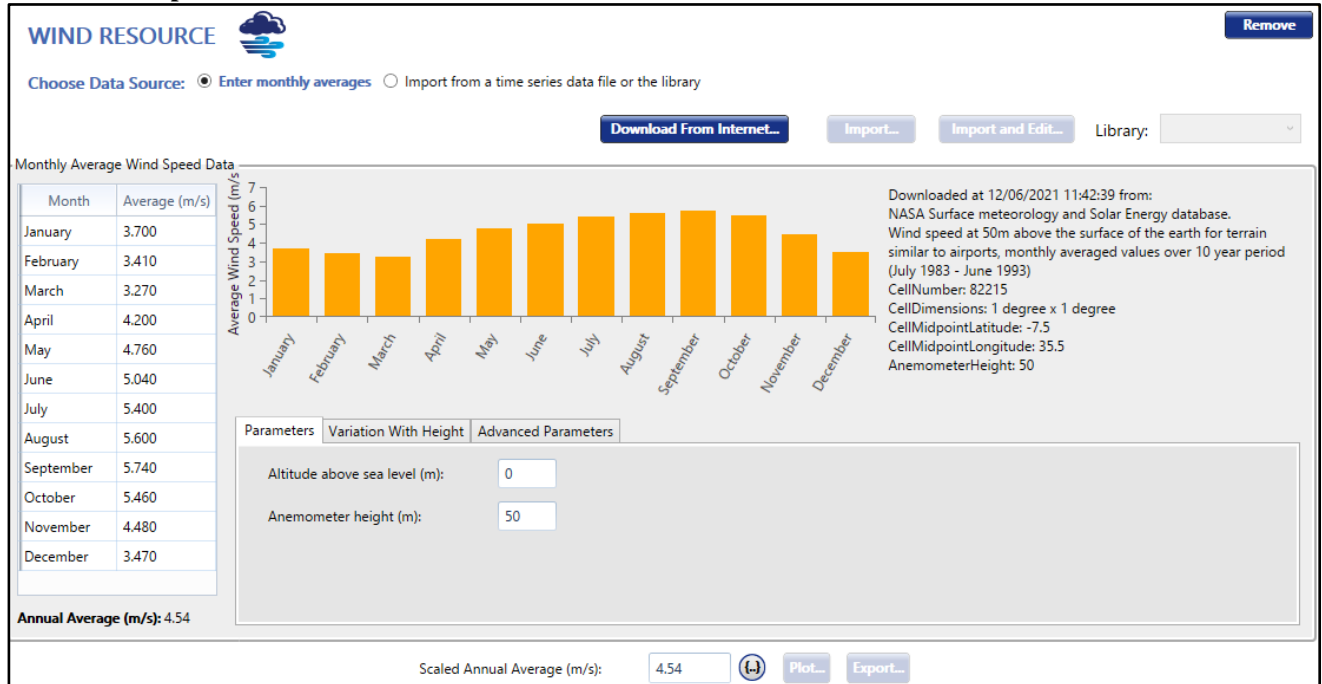
Figure 5: Monthly average Wind Speed data at Izazi, Tanzania
