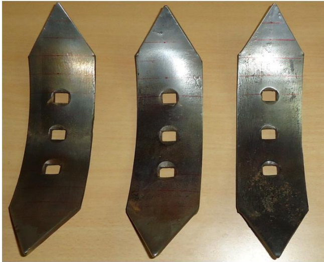
Fig. 6. Shovel with different substrate temperature coating after 100 hrs of working period.
