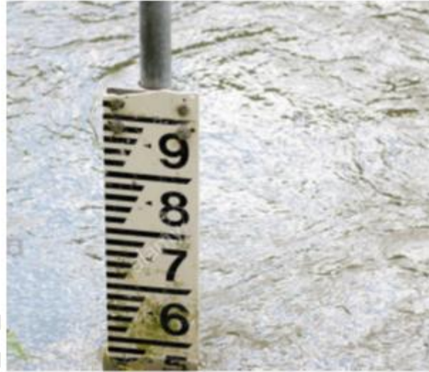
Fig. 9. Measuring canal depth with staff gauge
