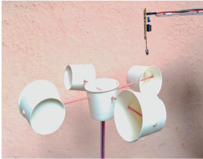
Fig. 15 IR sensor positioned with Anemometer
