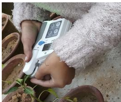
Fig: 1 Estimation of chlorophyll content of Capsicum annum using SPAD meter
