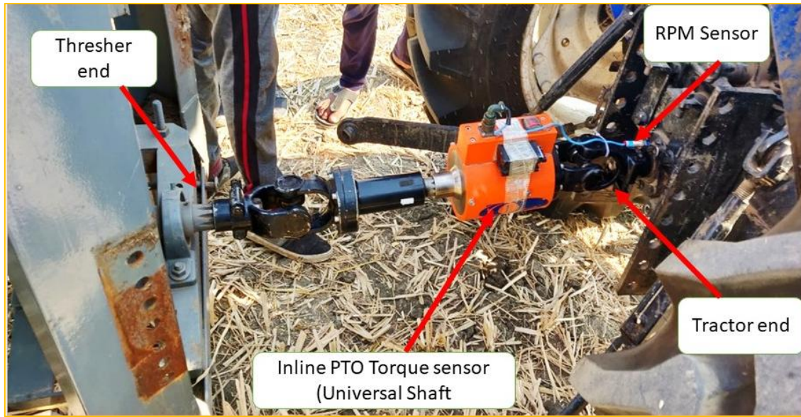
Figure 2 A view of in line torque sensor
