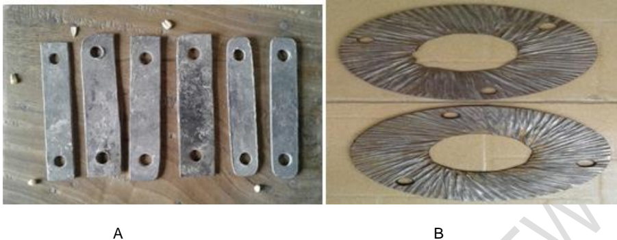
Figure 3: Grinding Machine Discs: (A) Hammer plates; (B) Disc plates
