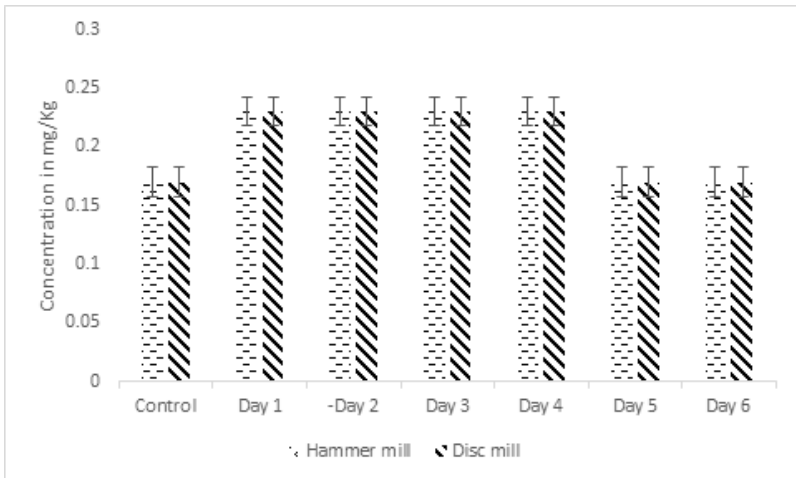
Figure 7. Ni concentration in maize flour milled with hammer mill and disc mill
