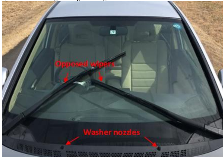
Fig. 16. Opposed pattern wiper blade of Honda Civic [16]
