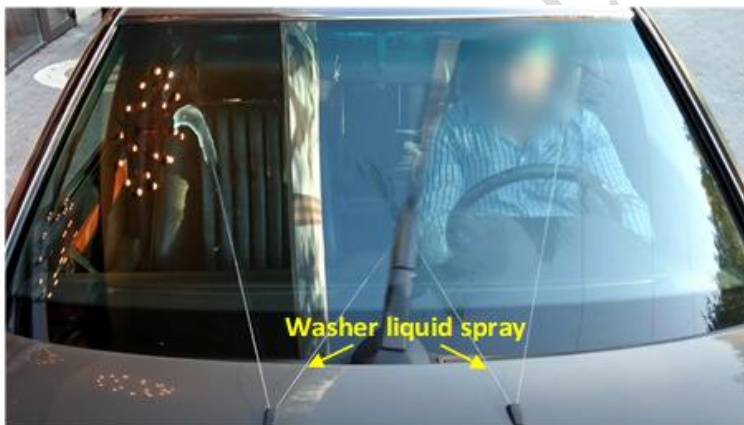
Fig. 10. Washer nozzle function of Mercedes-Benz W124 [11]
