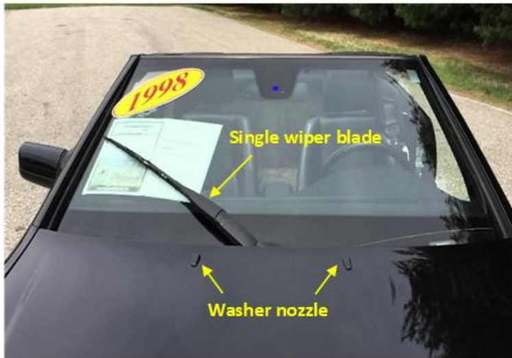
Fig. 9. Mono wiper blade of Mercedes-Benz W124 [10]
