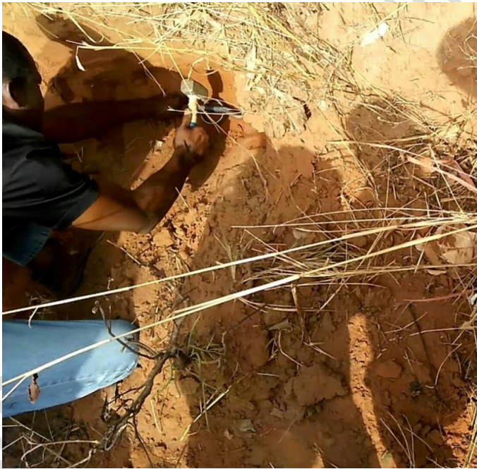
241 242 Fig 5a: Extracting Soil Sample with Core
