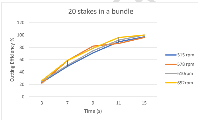
Figure 8. Effect of time on efficiency for various cutting speeds
