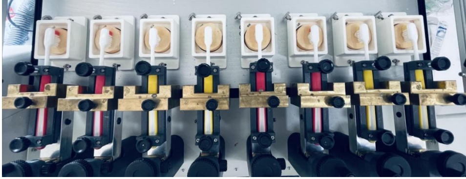
Figure 2: Image showing the subjecting of the two brands of GIC to standard and herbal toothpastes in a brushing simulator.
